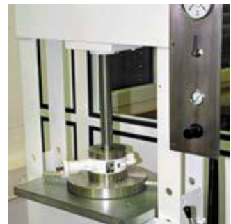
Tightness test with HP nitrogen
