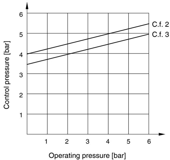
The control pressure depending on the prevailing operating pressure, as shown in the diagram, is intended as a guide for operating the system with low wear on the diaphragm.
